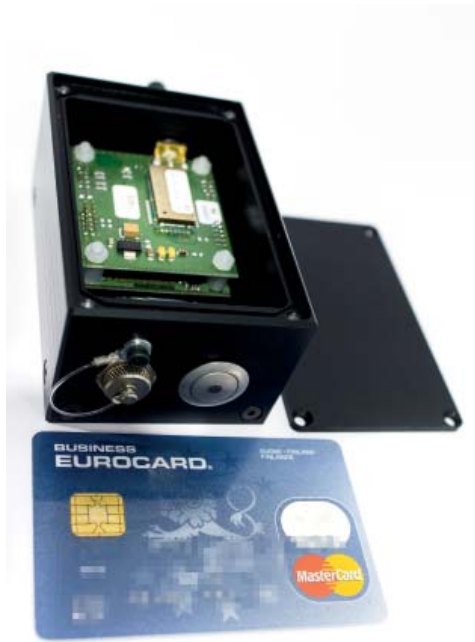
Figure 1. The prototype of the VTT Node has been installed in a robust casing and it has been used in several industrial demonstrators for vibration measurement purposes.
