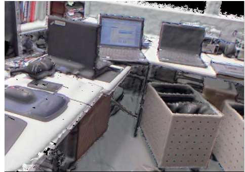
Figure 3. 3D reconstruction of an office room, based on depth sensor data. The aligned RGB image frames are used to combine the colour information in the scene.
