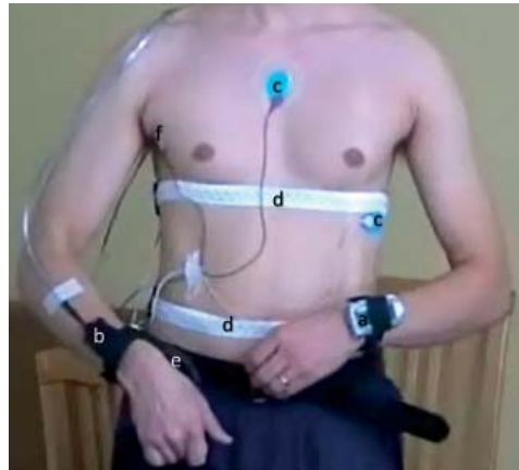
Figure 1. Combination of sensors used for assessing physical activities and mental load: a) audio recorder, b) 3D acceleration sensor box, c) two ECG electrodes, d) two respiratory inductive plethysmogram (RIP) belts, e) sensor box on the belt (acceleration, compass, light, humidity, and temperature sensors), f) skin temperature sensor.
