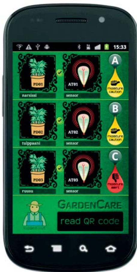
Figure 5. The gardener uses a smartphone that reports the moisture values and gives alarms if needed. The phone also provides the moisture threshold values and gardener presence information for the plant sticks via the M3 SIB.
