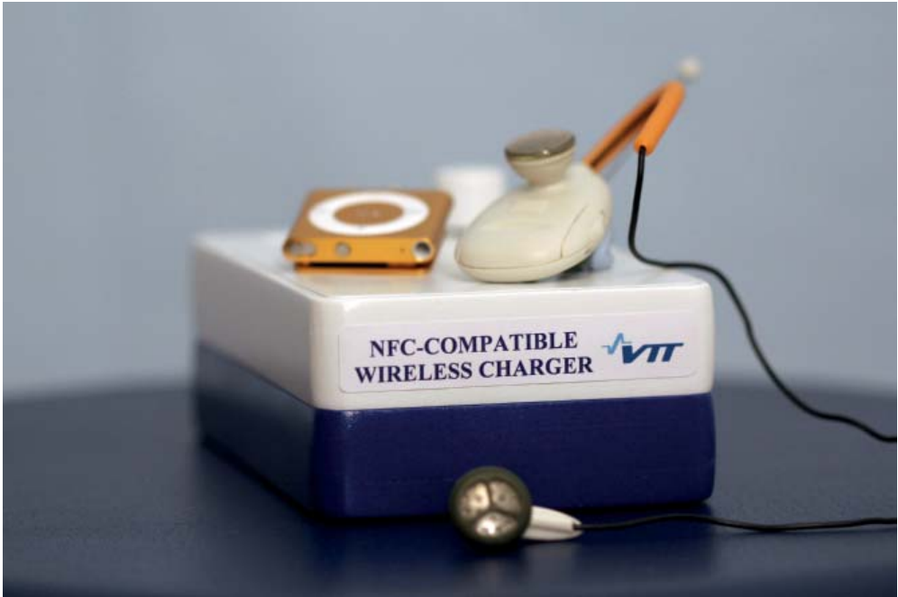
Figure 4. Demonstrator prototype of the NFC-compatible wireless power transmitter.
