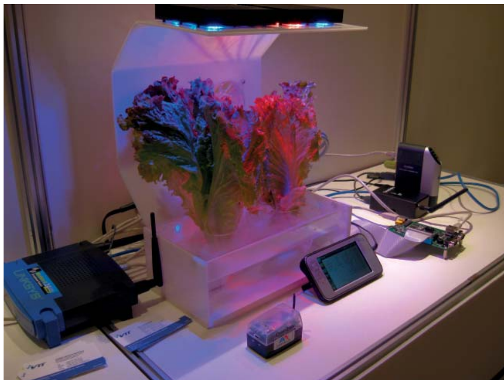
Figure 3. The Smart Greenhouse demonstrator is an example of an incrementally developed system consisting of autonomous devices and shared information-based interoperability.
