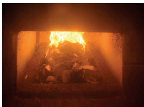
Figure 3a. 40 kW combustion chamber with mechanical grate used in the experiments.
