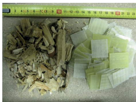
Figure 3b. CNT-containing composite and wood chips used as a supporting fuel for combustion.
