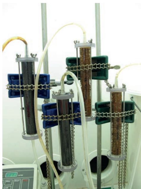
Figure 3. Column testing of sorption materials for the removal of arsenic from mine water.
