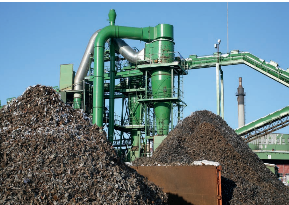
Figure 3. Hammermill shredding in large-scale operation at Kuusakoski's Heinola recycling plant. Shredded recovered metal is graded and sorted according to its elemental composition. Image courtesy of Kuusakoski Oy (Hanna Pynnönen).
