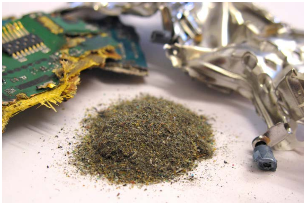
Figure 1. Electronics components and dust generated in the crushing process.
