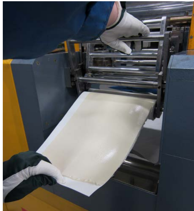
Figure 1. ATO-free PVC coating in a lab scale testing phase: sample preparation in a two-roll mill.
