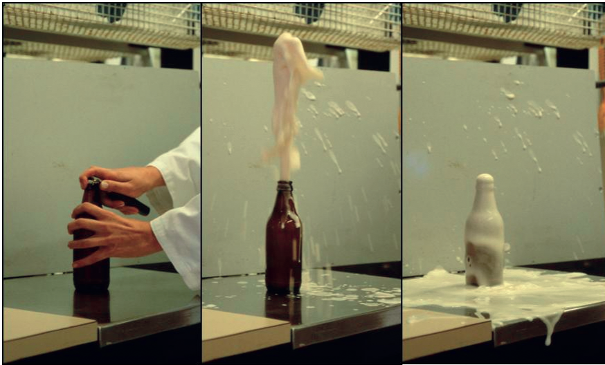
Figure 3. Gushing positive sample determined with the Carlsberg gushing test (Linder et al. 2005).
