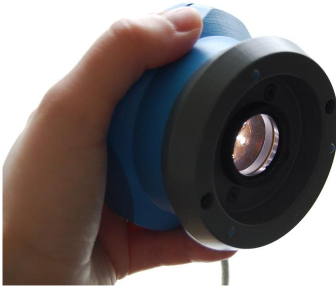
Figure 69. MEMS FPI ( \lambda = 500 \text{ nm} ) miniature imaging spectrometer [4].
