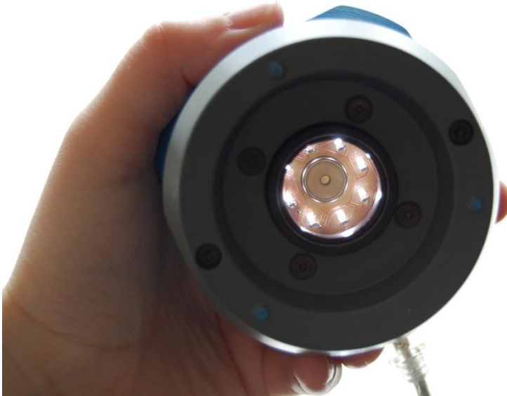
Figure 70. Inside of the imaging spectrometer showing the LEDs that illuminate the object as well as the packaged MEMS FPI aperture in the middle.
