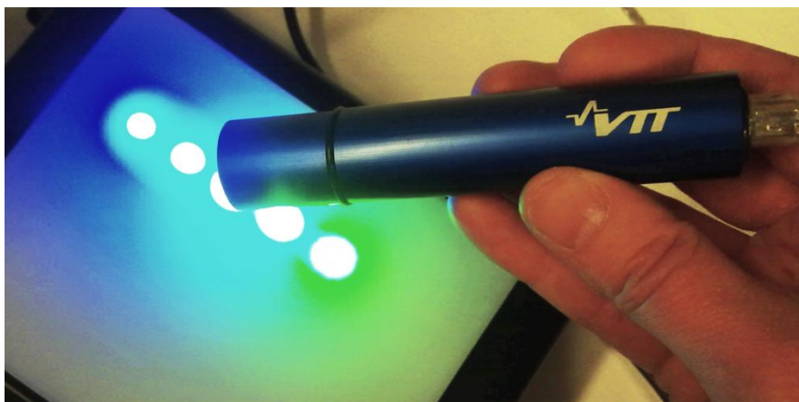
Figure 71. Pen-size spectrometer with \lambda = 500 nm MEMS FPI for single-point spectral measurements [4].
