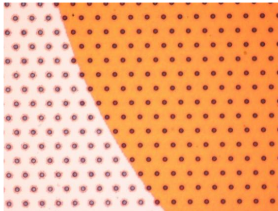
Figure 58. The membrane before release in oxygen plasma, showing the optical aperture area and the metal electrode. Red photoresist is visible in the open etch holes.
