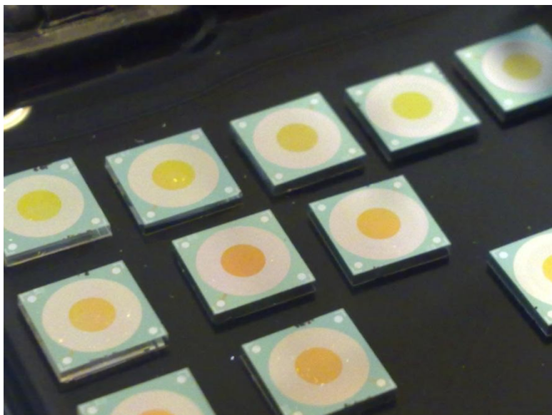
Figure 63. Completed and released MEMS FPI chips for \lambda = 670\text{ nm} .
