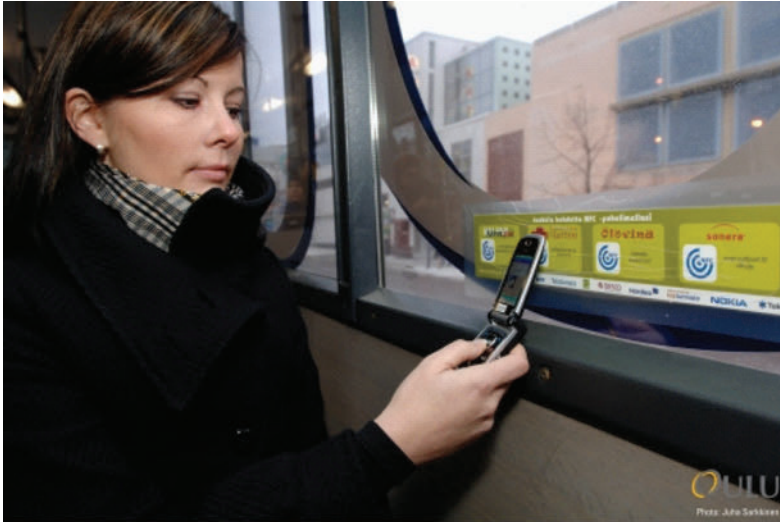
Figure 1. A passenger accessing Mobile Internet content through information tags available in a bus. Note that the symbol indicating the area to be touched is different in this version of information tags. It was later changed into an N-like symbol visible in the other figures.
