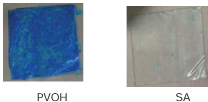
Fig 16. Colorant fixing to PVOH and lack of fixing to SA latex films after 30 s absorption time.
