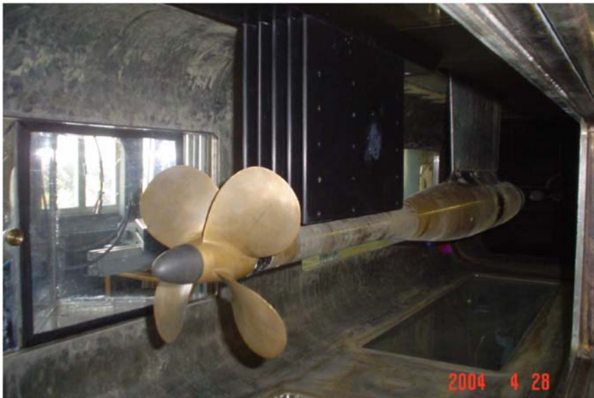
Figure 18. The INSEAN E779A propeller and the wake generator mounted in the cavitation tunnel of CEIMM. (Photograph is courtesy of CNR-INSEAN.)
