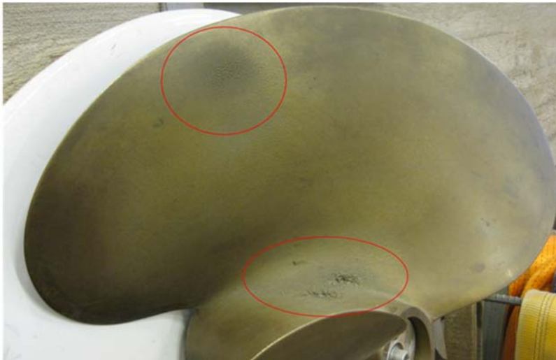
Figure 6. Cavitation erosion damage caused by root cavitation and cavitation cloud collapse near the trailing edge of a propeller blade.
