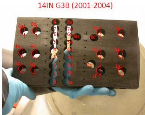
Figure 4.5. The tile 14 IN G3B exposed in 2001–2004 and the drilled sample locations used in tritium analyses.
