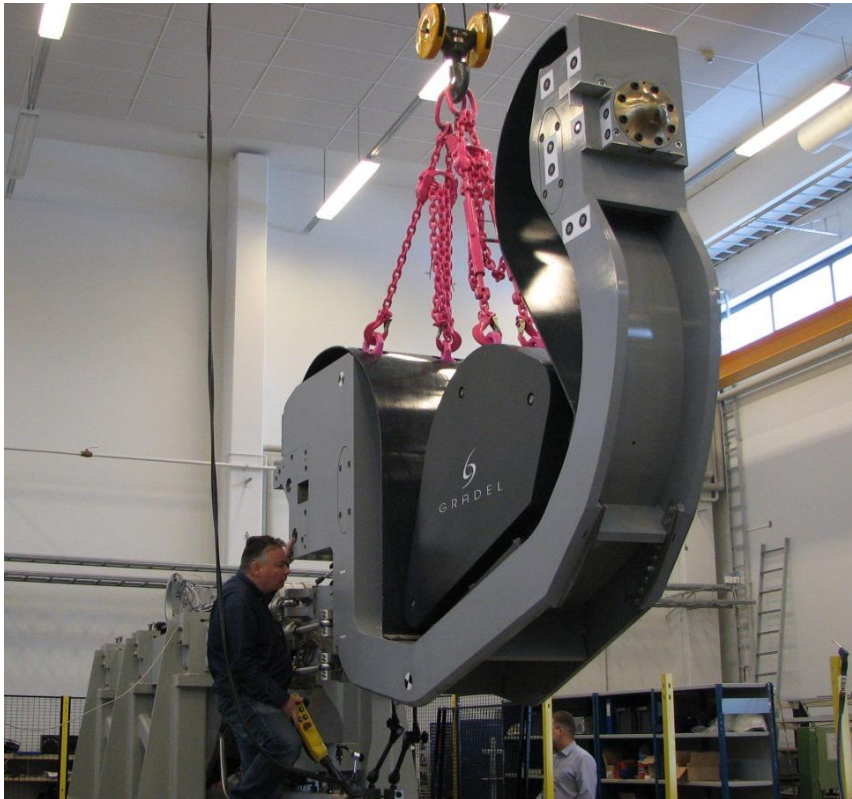
Figure 6.1. Testing the refurbished SCEE in the test stand after modifications.
