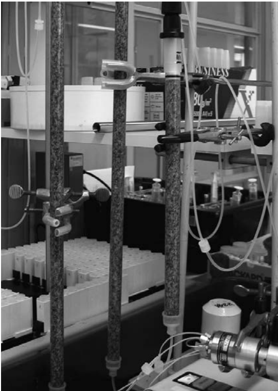
Fig. 1c. Experimental design used in core column experiments. Cores drilled to the fracture of the Kuru Grey granite, are placed inside a tube to form an artificial flow channel in a gap between the core and the tube.
