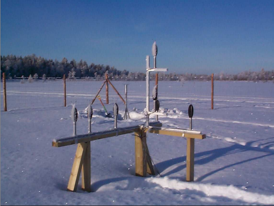
Fig. 3.5: The acoustic antenna with seven weather-proof microphones. There is a 2D sonic behind the acoustic antenna.
