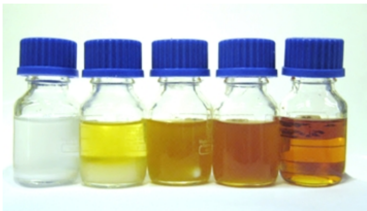
Figure 10. MCC (1% w/v) dissolution in [EMIM]AcO/buffer (45 °C, 1 d mixing) as a function of [EMIM]AcO concentration. From the left: buffer, 20, 60, 80 and 90% (v/v) [EMIM]AcO in buffer. Note that the bottles also contain a magnetic stirring bar.
