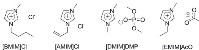
Figure 5. The most studied cellulose-dissolving imidazolium-based ILs: 1-butyl-3-methylimidazolium chloride ([BMIM]Cl), 1-allyl-3-methylimidazolium chloride ([AMIM]Cl), 1,3-dimethylimidazolium dimethylphosphate ([DMIM]DMP) and 1-ethyl-3-methylimidazolium acetate ([EMIM]AcO).
