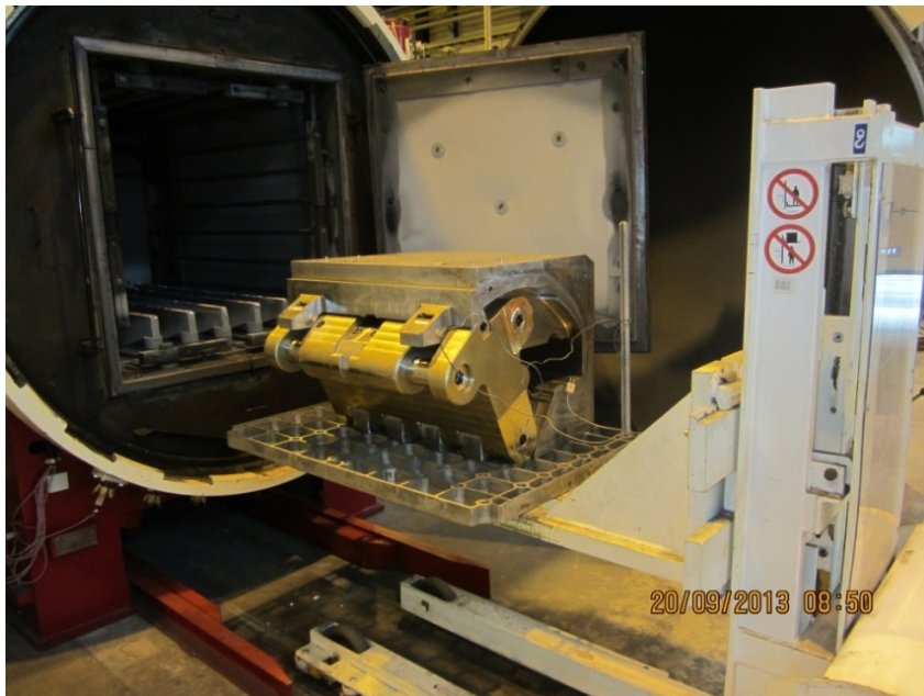
Figure 5.3. Cassette locking system after heat treatment in a vacuum furnace.
