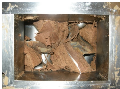
Figure 4. Bran mixture at a water content of 40% in a Farinograph mixer after 24 h treatment with xylanase enzyme preparation Depol 761P (20 nkat/g) (Publication I).
