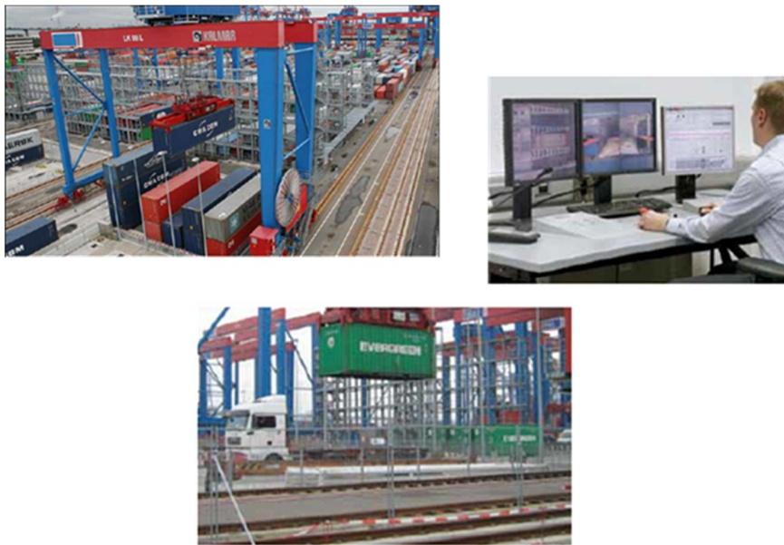
Figure 32. Pictures of the ASC in operation at HHLA's Burchardkai container terminal, in Hamburg (Cargotec). Figure used with permission from Cargotec.
