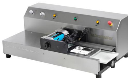
Figure 20. Laboratory-scale sheet-based gravure printing machine (Schläfli Labratester I).
