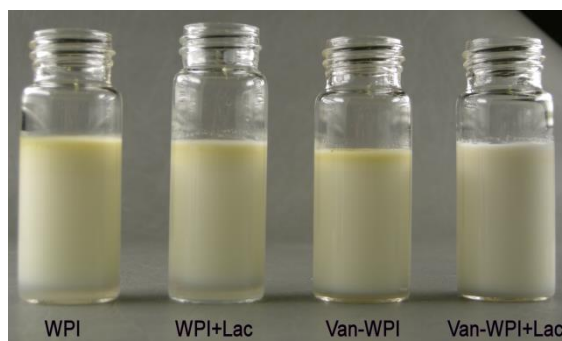
Figure 11. Visual observation of aged emulsions. The emulsion samples were stored at RT for 1 week. Clarification and creaming were observed respectively from the bottom and the top of tubes.
