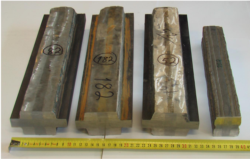
Figure 18. All-weld metal test blocks of Alloy 82, Alloy 182, Alloy 52 and Alloy 152, respectively.
