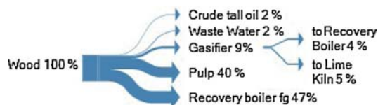
Fig. 5. Carbon flow in a typical modern integrated pulp and paper mill.
