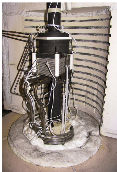
Fig. 2. The 30-cell stack before testing.
