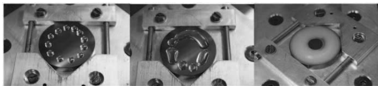
Fig. 2 HFBI of concentration 0.1 mg/mL on the disc before and after the test Note: The lubricant was added onto the disc by a syringe drop by drop and it did not spread to the whole disc surface. During the test, the lubricant changed its colour to white because of the protein agglomerates, as shown in the picture on right. The diameter of the discs is 40 mm
