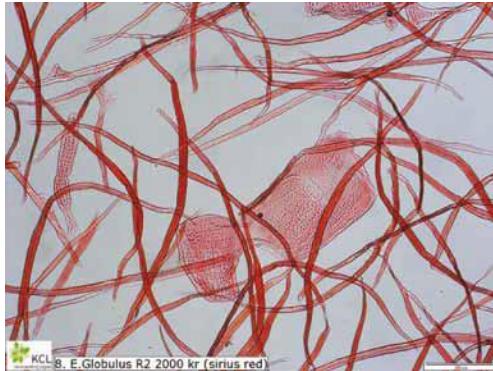
Figure 32. Refined vessel-rich fraction of Eucalyptus globulus pulp.
