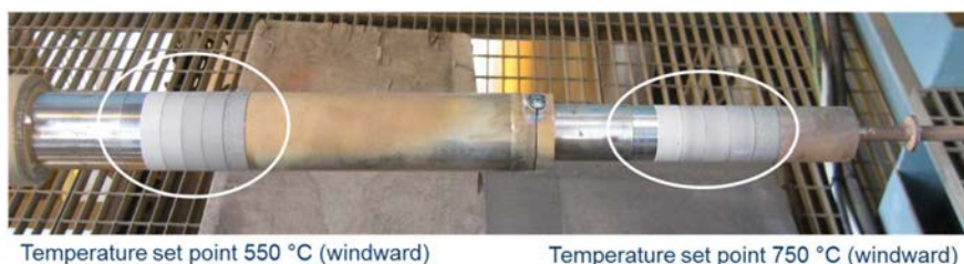
Figure 9 Test probe before exposure in a biomass co-fired boiler. On the left, section with specimens exposed to 550 °C; on the right specimens exposed to 750 °C (Ref 95).
