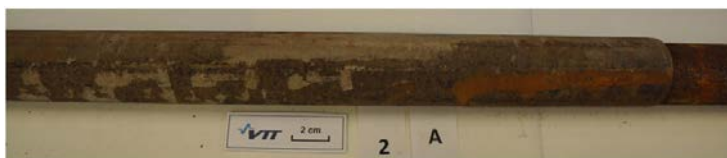
Fig. 8. A coated boiler tube after the exposure. Severe material wastage of the uncoated tube can be detected in the right side of the picture.
