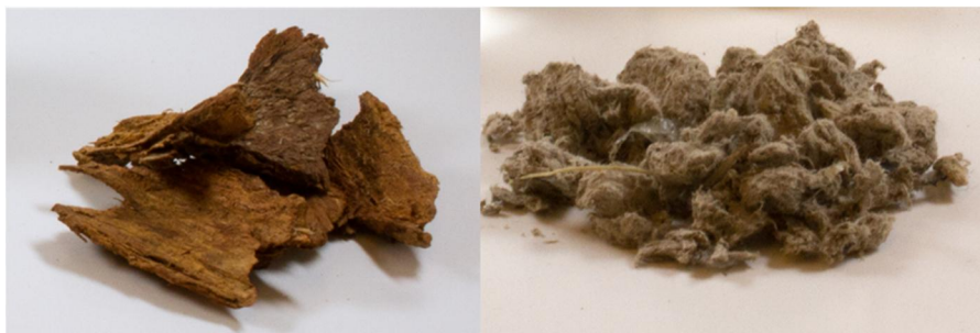
Figure 10. Spruce bark and recovered fibres fractionated from solid recovered fuel.
