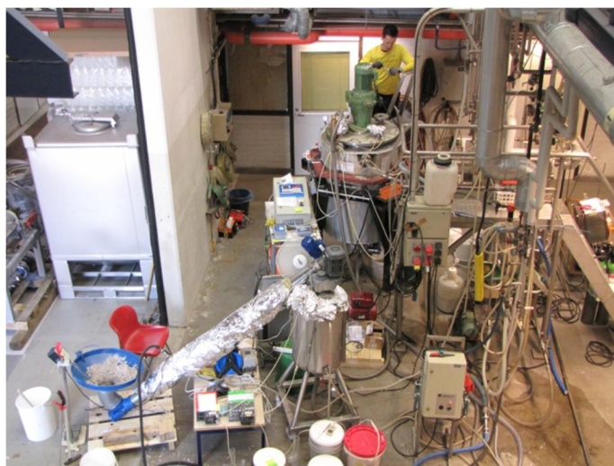
Figure 17. Schematic view of the pilot process and a photograph of the same set-up. SL) screw lift, H) prehydrolysis tank, F) fermenter.
