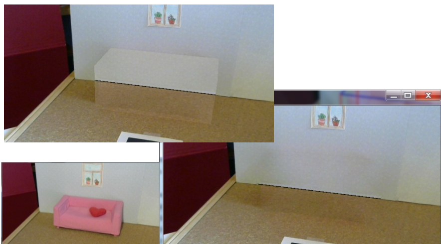
Figure 44. Frames without (top) and with (bottom) adaption to current illumination; the small image shows a frame before diminishing. The inpainting texture was created from a lighter frame.
