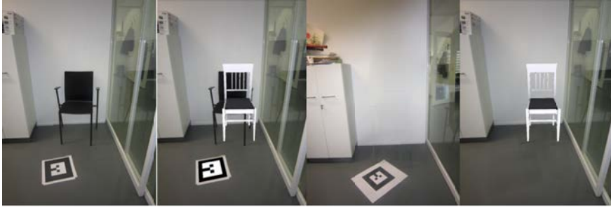
Figure 12. Example of diminished reality. Left to right: original image; augmentation over existing object; diminished image; augmentation over diminished image (Siltanen 2012).
