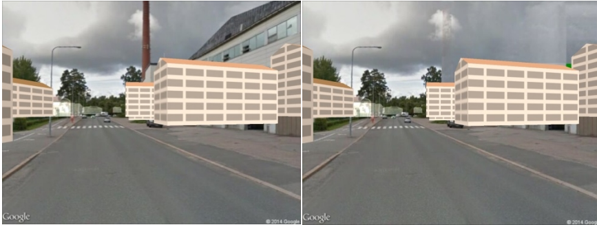
Figure 54. An example of using diminished reality in an AR application for construction visualization. On the left, the buildings to be demolished disturb the AR visualization of the new construction plans. On the right, the visualization result is clearly improved through diminished reality.
