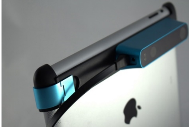
Figure 58. StructureSensor attached to an iPad. (Image source: StructureSensor.)
