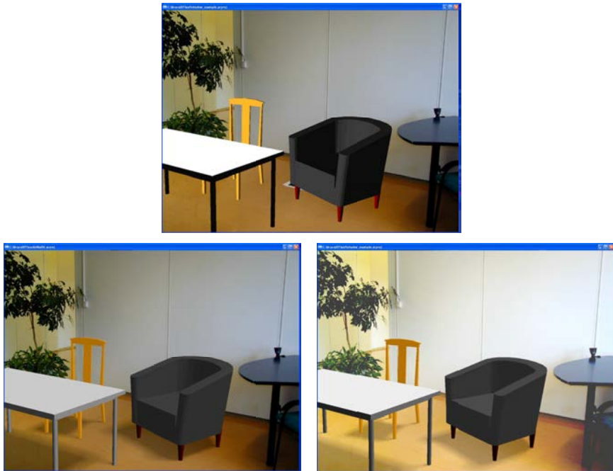
Figure 31. Augmentation without adaptation (top) and with adaption under two different illumination conditions (below).
