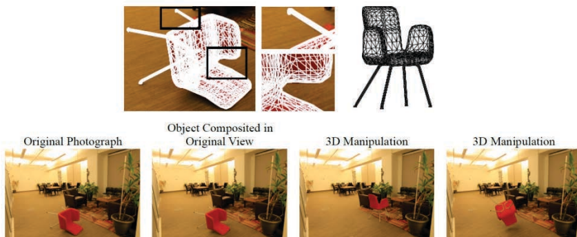
Figure 59. A 3D model is positioned and adjusted over an object in a photograph. Thereafter the object can be moved and rotated freely, as if it were 3D graphics. Images from (Kholgade et al. 2014).
