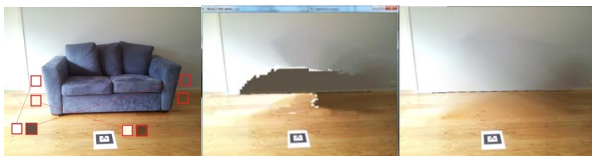
Figure 47. Our solution can handle large illumination variations during initialization of inpainting texture. Images from left to right: Original image, inpainting without texture normalization, inpainting with texture normalization.
