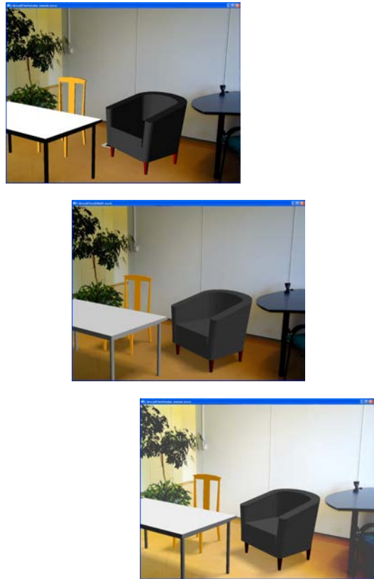
Figure 4: Without shadows, virtual objects seem to hang in the air, and if virtual lights are fixed, the brightness of objects is often unnatural (top). We augment virtual soft shadows underneath virtual objects and enable adjusting the virtual lights to the real room lighting (middle and bottom).
