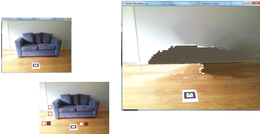
Figure 39. Example of problems with exemplar-based inpainting with a strong contrast image where samples of intermediate darkness are rare. The small images show the original image (cf. Figure 47 where normalization is used).
