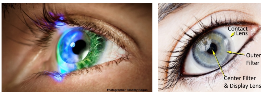
Figure 57. AR contact lenses by Innovega. (Left image: Timothy Hogan.) Images courtesy of Innovega.
