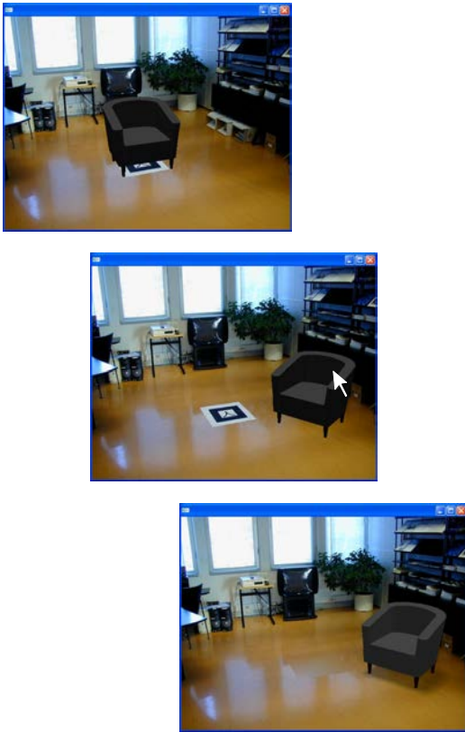
Figure 3: (Top) virtual object placed over the marker, (Middle) object moved and rotated to desired position (Bottom) marker erased and shadows added.
