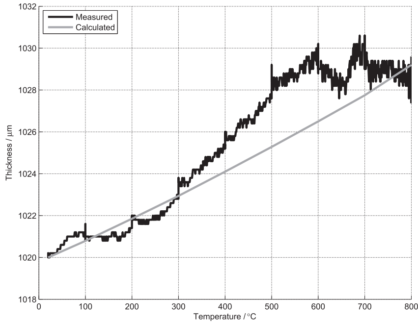
Fig. 2. Measured thickness of Crofer 22H plate (1020 \mu\text{m} initial thickness) as a function of temperature together with calculated thickness based on manufacturers datasheet.
