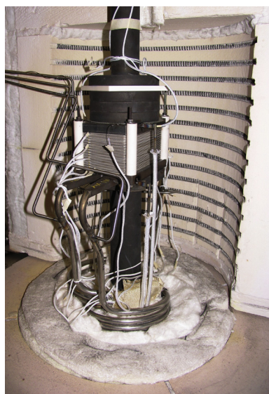
Fig. 2. The 30-cell stack before testing.
