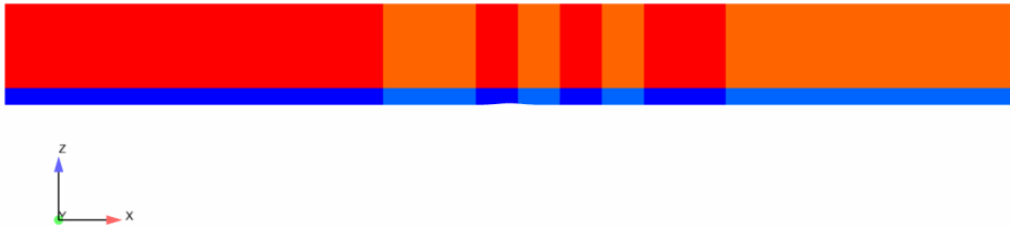
(a) Overview of the block division of the coarser grid. The blocks initially above the free surface are coloured with red, and those initially below it are coloured with blue. The different shadings distinguish the blocks.
