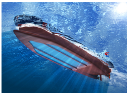
(d) An example of air cavities to reduce the frictional drag.
