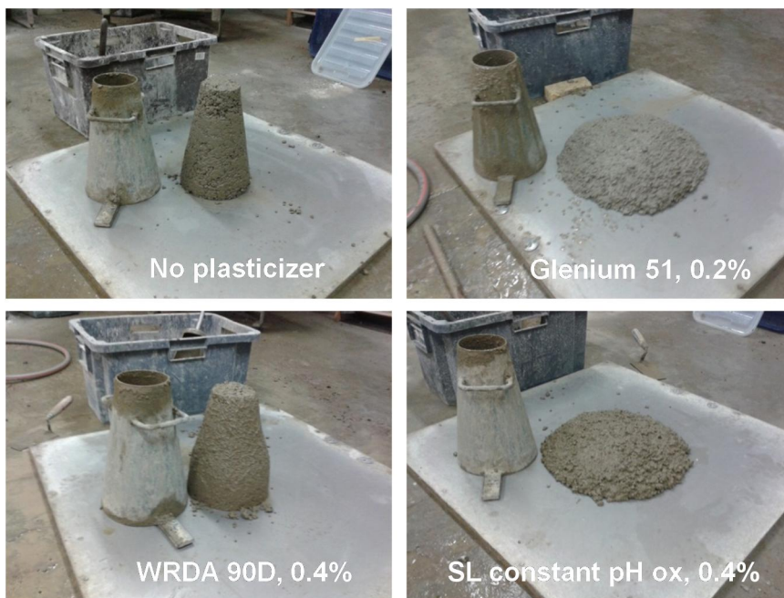
Figure 20. Photos of the concrete slump test. Commercial products (Glenium 51, WRDA 90D) or an oxidized soda lignin solution (SL constant pH ox) used as plasticizers, with dosages of 0.20 and 0.40 w-% on cement.
