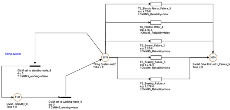
Fig. 89 - Tilting system of the CMM (electrically actuated)
