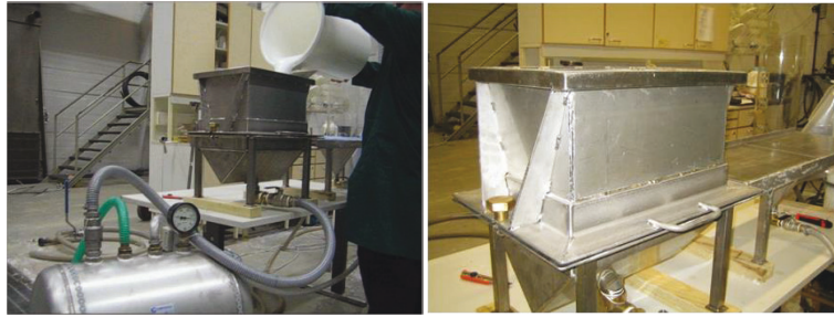
Figure 2. The foam forming handsheet mould and the equipment set-up.
