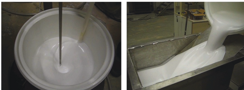
Figure 19. The procedure of the foam laid handsheet making. (1) An aqueous fiber suspension is mixed with a prefabricated foam produced from water and sodium dodecyl sulphate (SDS) in ratio 0.15-0.20g/L. (2) The fiber foam is decanted into the handsheet mould and filtrated through a wire using a vacuum chamber. The sheet is pre-dried on a suction table (0.2 bar vacuum).
