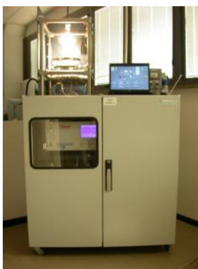
Figure 1. The photodegradation kinetics of \text{NO}_x in gaseous phase by foam-coated papers were tested using a photo-reactor equipped with chemiluminescence and GC/MS by Colorobbia (Italy).
