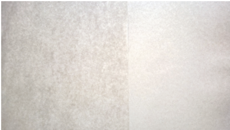
Figure 45. Comparison of formation from the samples run at the KCL pilot paper machine using water and foam forming techniques, the Ambertec beta radiation values and the images correspond to the values. Top: The specific formation, bottom: A picture from the sheets; water formed (left) and foam formed (right). The water formed sample consist of refined SW and HW pulps (30/70), and the foam formed sample unrefined SW and PP fibers (70/30). PP fiber fraction was a mixture of 6 and 12 mm fibers (50/50).
