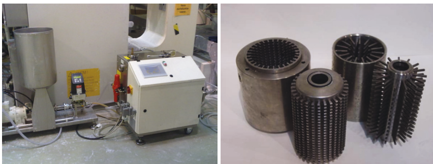
Figure 14. The foam generator (left) and examples of the mixing head's rotor-stator sets (right).
