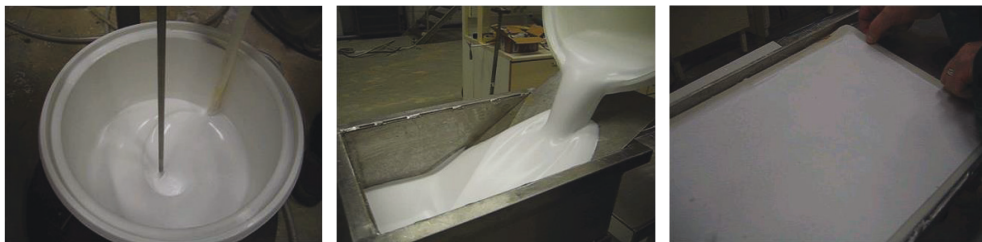
Figure 3. The procedure of the foam laid handsheet making. (1) An aqueous fiber suspension is mixed with a prefabricated foam produced from water and sodium dodecyl sulphate (SDS) in ratio 0.15-0.20g/L. (2) The fiber foam is decanted into the handsheet mould and filtrated through a wire using a vacuum chamber. (3) The sheet is pre-dried on a suction table (0.2 bar vacuum).
