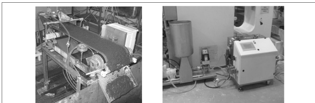
Figure 4: The dynamic setup comprised of a dynamic thickening unit (left) and a foam generator (right).
