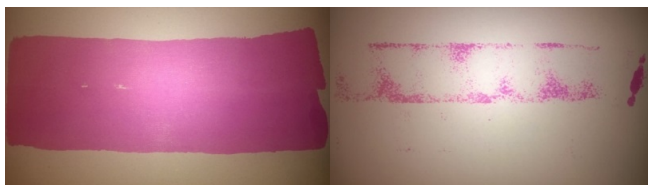
Figure 2. Pinhole test. A coloured oil is applied onto the surface (left). The penetration is observed from the opposite side (right).
