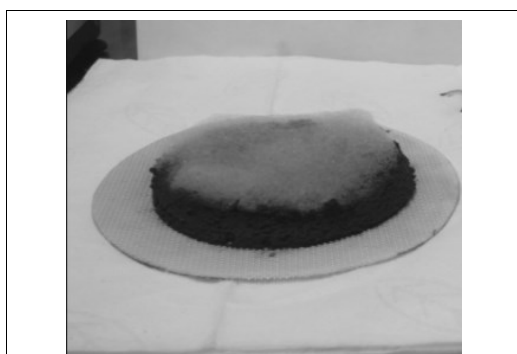
Figure 3: An example of the filter cake produced by using a foam-assisted thickening technique in the treatment of biosludge from a paper mill.
