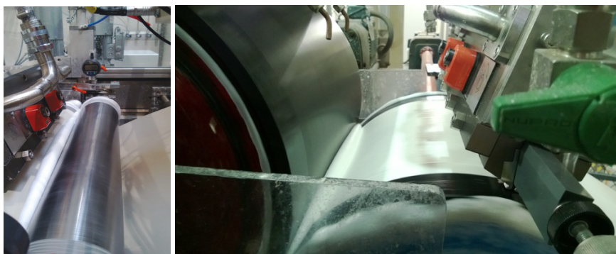
Figure 17. In the contact foam coating method, the foam is applied as a foam curtain, but the foam destruction is accomplished with nip pressure. The left nip arrangement with small rolls is from the VTT line used in the thesis' trials. The right picture is an example from the customer trials.
