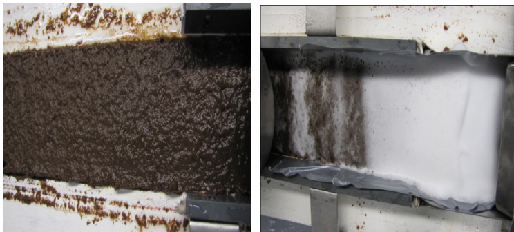
Figure 60. An example of the sludge web before (left) and after applying foam (right) in the dynamic filtering process.
