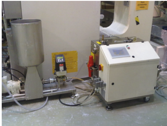
Figure 22. The dynamic set-up consists of a dynamic thickening unit and a foam generator.
