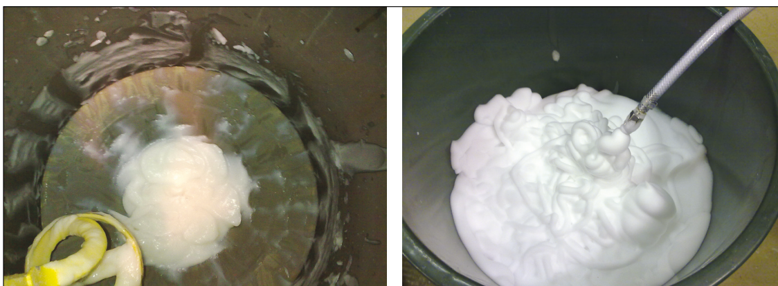
2. Cellulose nanofibrils (CNF) with solid content 2.9 % (left), and foamed CNF containing 90% air (right).
