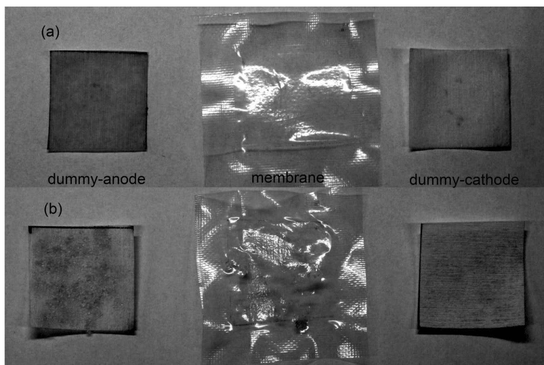
Figure S2. Colored DI-water on clean room paper placed in closed test cell (a) without and (b) with superabsorbent polymer. The cells were kept assembled for 24 h.
