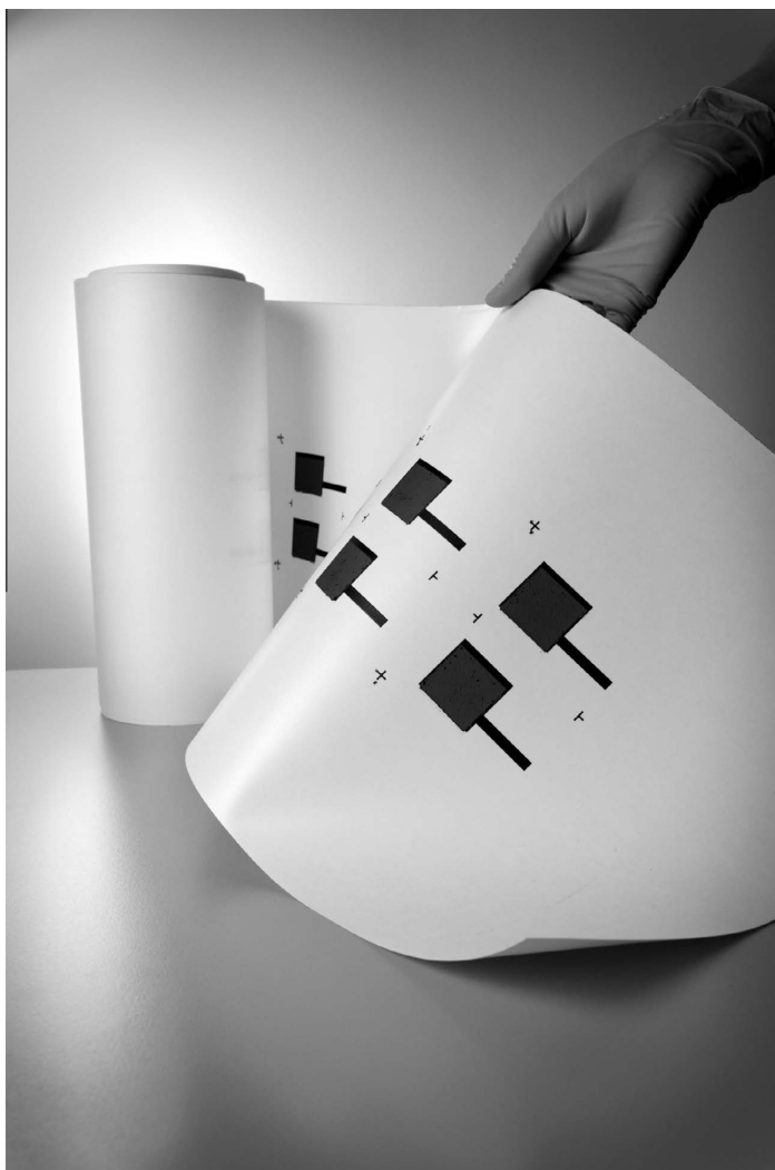
Fig. 2. A roll of printed bioelectrodes on cardboard.
