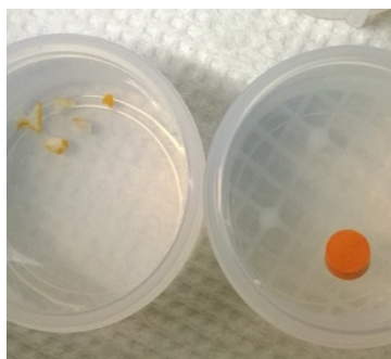
Figure 9. A Picture of the ^{229}\text{Th} tracer experiment with fragments and a single pellet of \text{ThO}_2 .
