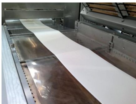
Figure 25. A smooth layer of pigment-CNF dispersion was spread on top of the support material.
