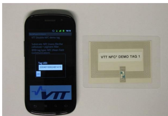
Figure 38. An image of a screen-printed antenna combined with a commercial RFID chip as demonstrator of an RFID tag manufactured on PCMNf composite. The device has been hot-laminated into a plastic pocket. The content of the tag can be read with a mobile phone supporting NFC technology.
