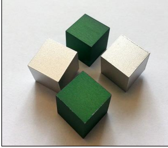
Figure 10. Anodised and non-anodised roughened aluminium surfaces. The dimensions of the cubes are 12 mm x 12 mm x 12 mm. In order to avoid the edges from rounding, the roughening process was performed for multiple samples at once, with the sides of the cubes tightly adjacent to each other.
