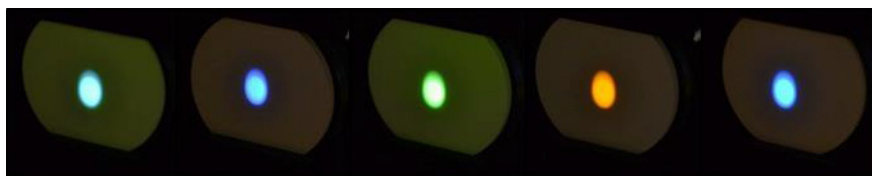
Figure 16. A set of PTFE based photoluminescent materials illuminated at the wavelength of 380 nm in the MIKES-Aalto goniofluorometer.
