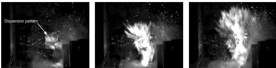
Fig. 15. Far-field liquid dispersion pattern from 3D projectile test no. 695 with an impact velocity of 167 m/s and 8 L of water. The time instances are 1, 5 and 10 ms after the impact.
