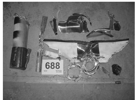
Fig. 11. A 3D projectile after test 688.
