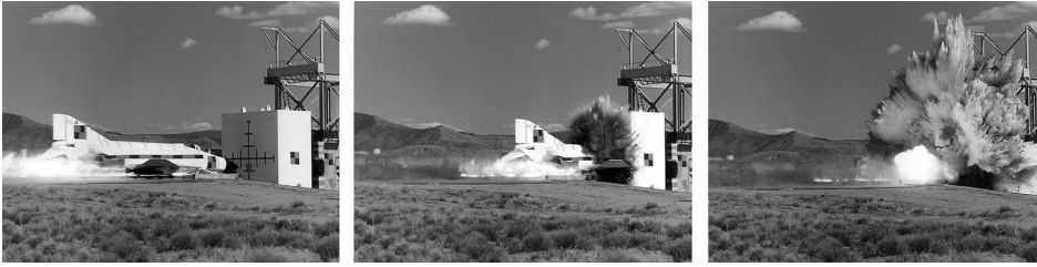
Fig. 1. Still figures from the video clips of the Phantom F-4 test by Sandia National Laboratories. From https://share.sandia.gov/news/resources/video-gallery/index.html#rocketsled (accessed 12.03.15).
