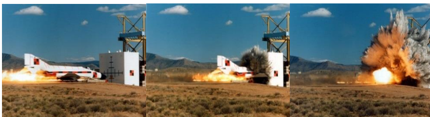
Figure 2.2 Still images from the video clips of the Phantom F-4 test by Sandia National Laboratories
