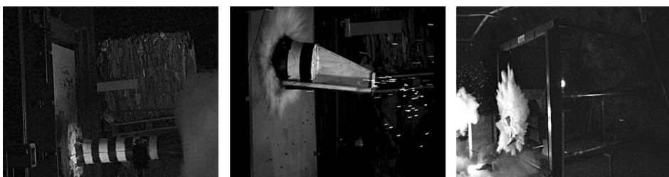
Fig. 16. Side view images of liquid dispersion pattern in selected VTT impact tests (note that each image is taken from different tests).
