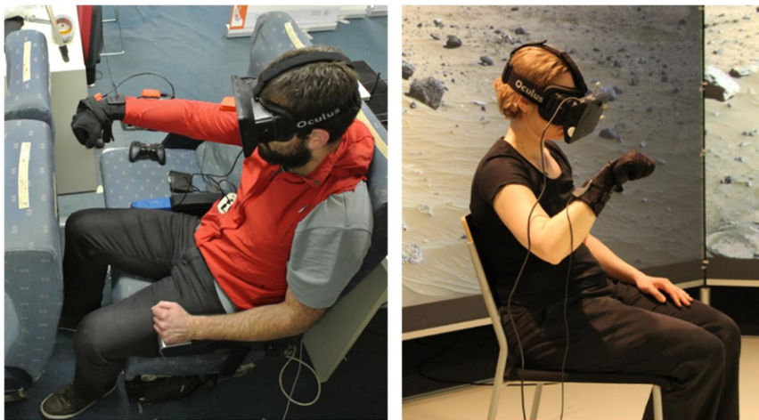
Figure 18. Gesture-based interfaces for robot control. The sensor-based system (on the left-hand side) and a computer-vision-based system (on the right-hand side).
