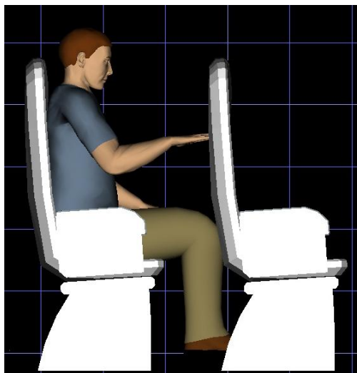
Figure 7. An example of a digital human model, Jack.
