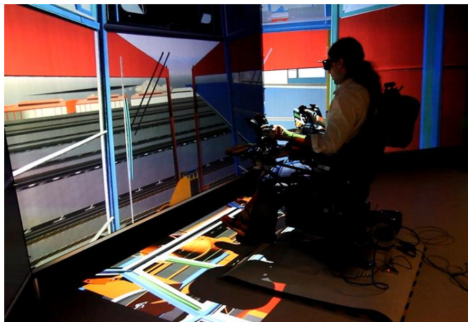
Figure 14. The user is performing a task using a virtual prototype of a crane.
