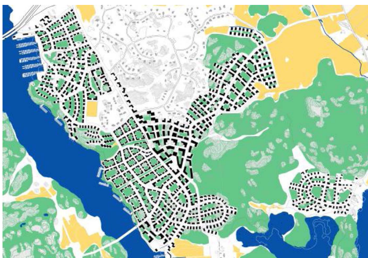
Fig. 4. Draft of the master plan of Eriksnäs (modified from Eriksnäs city plan, 2012). The drafted new building blocks under planning are shown with as black blocks (grey blocks are already existing in the area). Blue areas are sea, green areas are parks and leisure areas, and yellow areas are cultivation fields.
