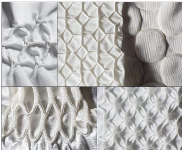
Fig. 8. Structures printed using cellulose dissolved in ionic liquid could be used for smocking effects (design: Pauliina Varis and Ilona Damski, photos: Eeva Suorlahti).
