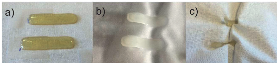
Figure S6 Photographs of the behaviour of dissolved cellulose in an ionic liquid a) after printing b) after regeneration c) after drying
