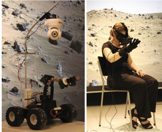
Fig. 1. Left: Robot system. Right: User with HMD and data glove in a mixed reality laboratory. The hand posture is IDLE.
