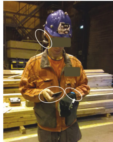
Figure 2. A maintenance technician using a wearable system for data collection and reporting.
