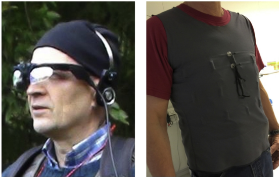
Fig. 1. Wearable devices. Left: HMD for presenting visual modality. The light-weight headphones were used in Study 1 and in the bimodal VA condition in Study 2. Right: Tactile vest showing three rings of tactors.
