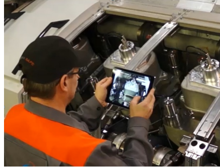
Figure 3. Maintenance technician using augmented reality system for task guidance.
