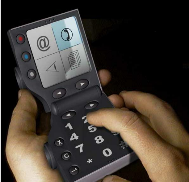
Figure 1. CyPhone has a 1:1 user interface because a touch-pad and a display screen have same size. The shape of left side is designed for bringing the mini displays near eyes.
