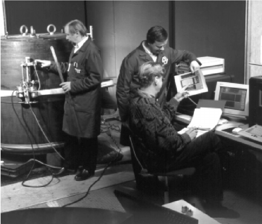
Figure 6. Inspection of the NESC cylinder with the mechanized ultrasonic equipment of VTT.
