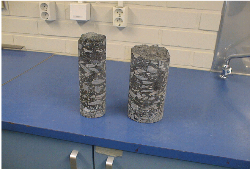
Figure 3. Two Ekostab-core samples taken from the road.
