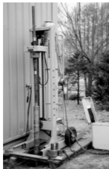
Photo 3. View of the shallow depth boring machine.
