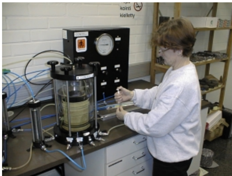
Figure 1. Water permeability is measured by the Concell-meter.
