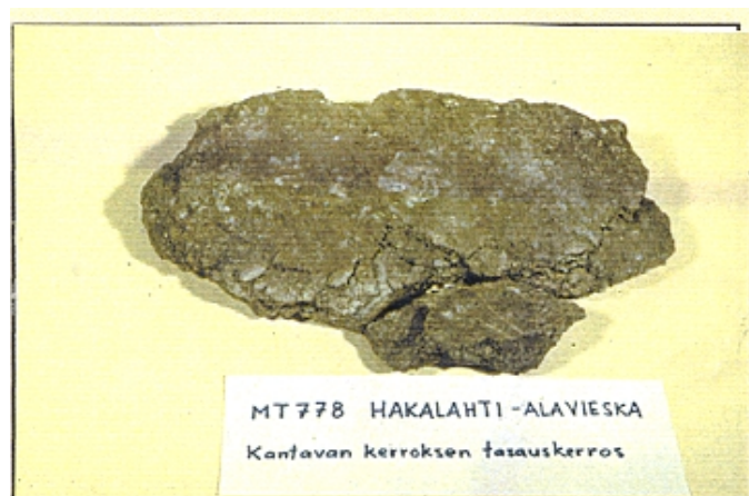
Figure 3. Use of crushed blastfurnace slag as a temporary surface during road construction work.
