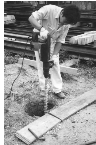
Photo 5. Surface soil sampling with electric hand drill.
