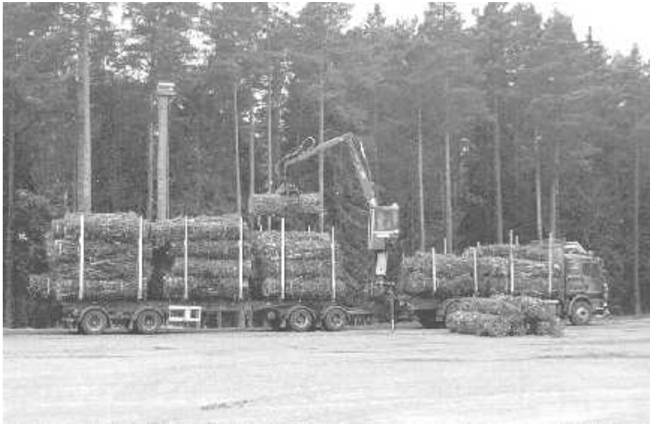
Figure 3. A conventional roundwood rig can accommodate some 66 CRLs – 15 per stack on the trailer and 10 or 11 per stack on the truck. A pulpwood bolt is placed on either side at the bottom of each stack to prevent the load from overhanging the load-securing devices.
