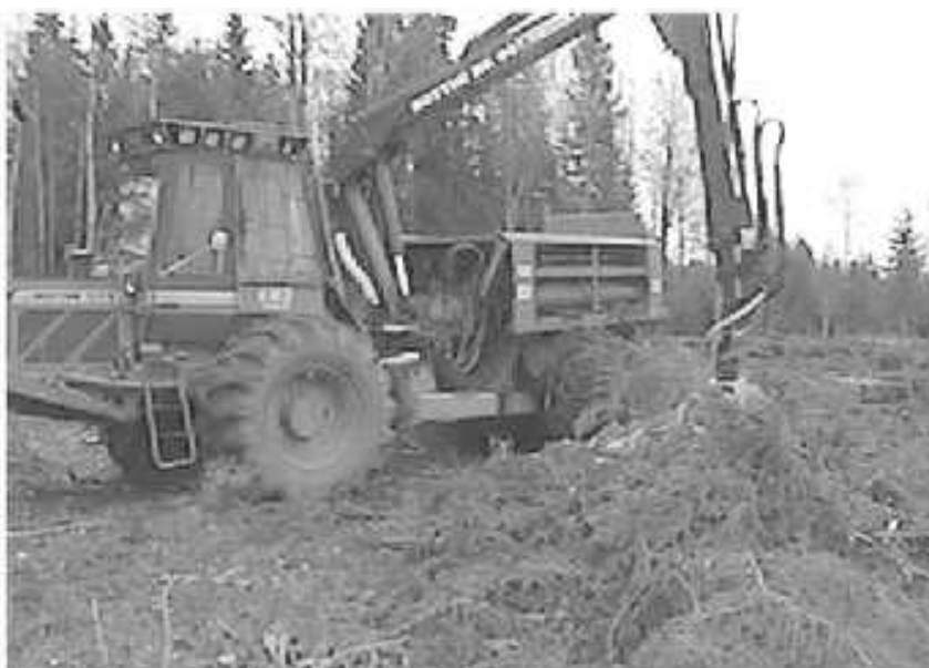
Figure 2. Wood Pac mounted on a Rottne forwarder. Compaction chamber consists of 8 cylinders and is topfed.
