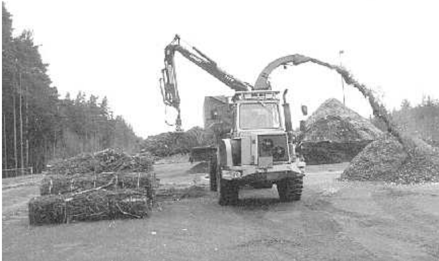
Figure 4. A Bruks 1004 CT drum chipper mounted on a dumper-truck chassis. This chipper has a capacity of 200,000 m 3 (solid) over an eight-month season and assuming a mechanical availability of 60%.
