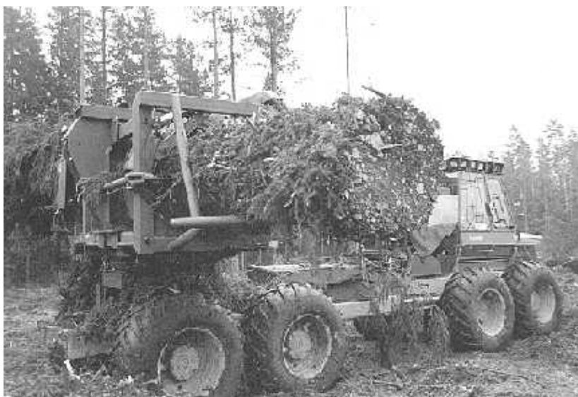
Figure 1. The Fiberpac 370 weighs approximately 6 tonnes and can be mounted on a medium or heavy-duty forwarder.
