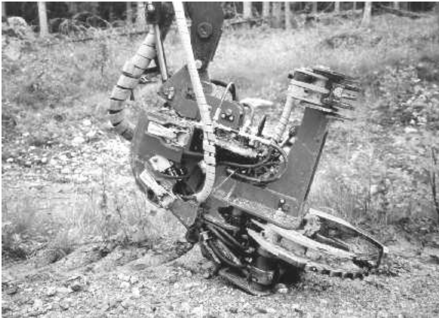
Figure 6. The EnHar unit – an accumulating or multitree-handling head for felling and baling.
