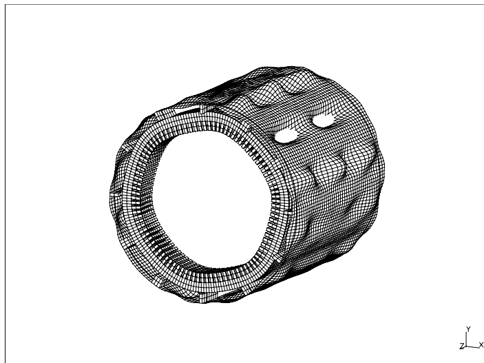
Figure 7. A local natural mode of the stator frame.
