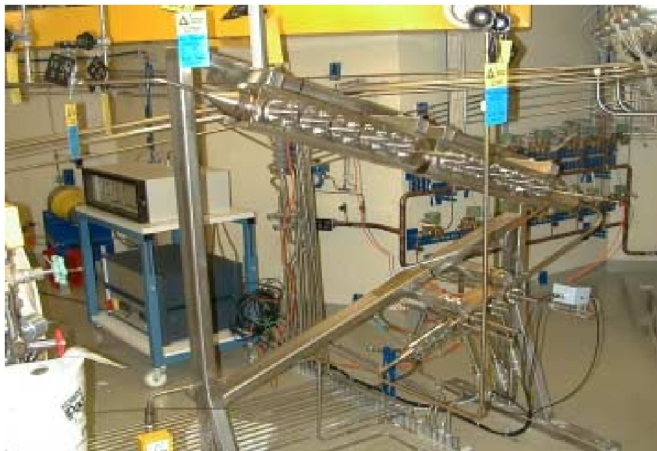
Figure 2. Flow-through cells with high temperature water chemistry sensors (lower cell) and 80 stainless steel samples (two upper cells) at Loviisa unit 1.
