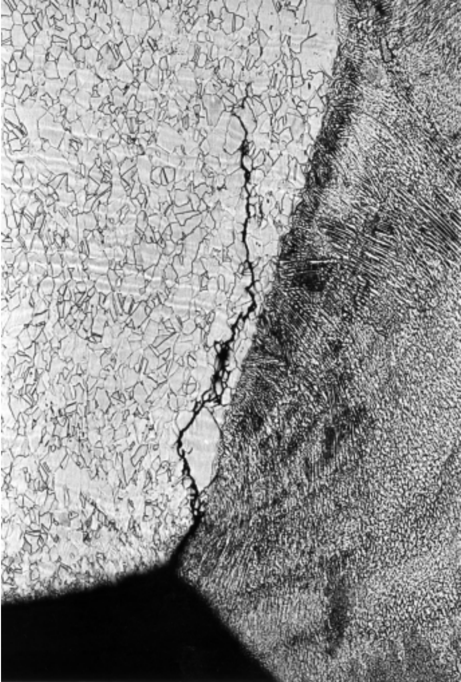
Figure 4. IGSCC in a non-sensitised, deformed AISI 316NG type stainless steel.
