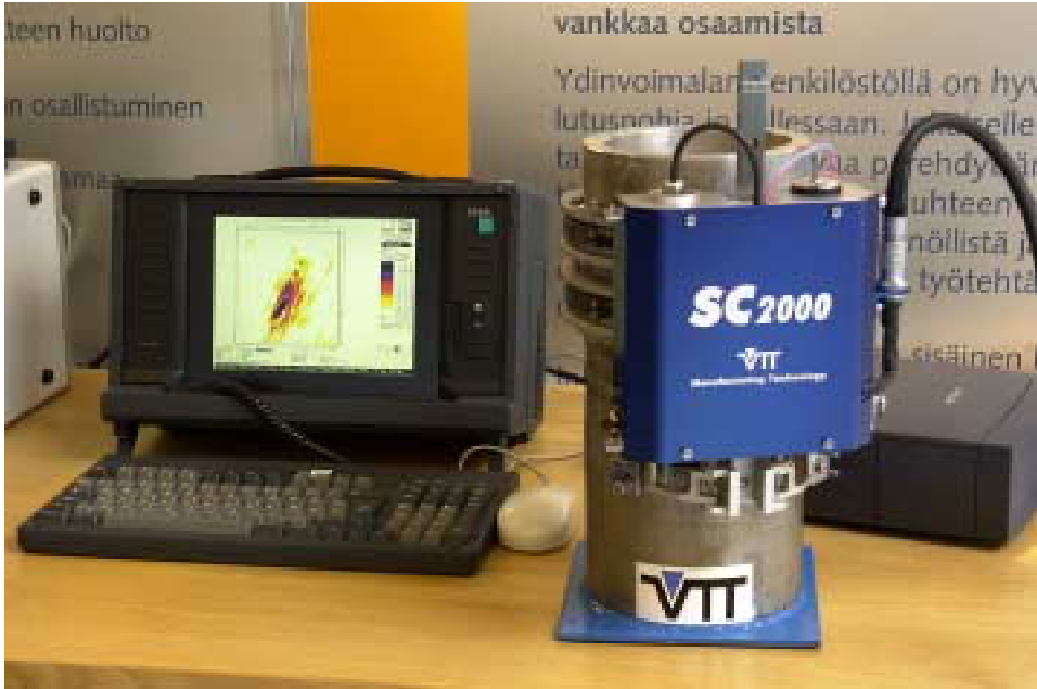
Figure 1. SC2000 scanner for mechanised ultrasonic inspection of pipings.
