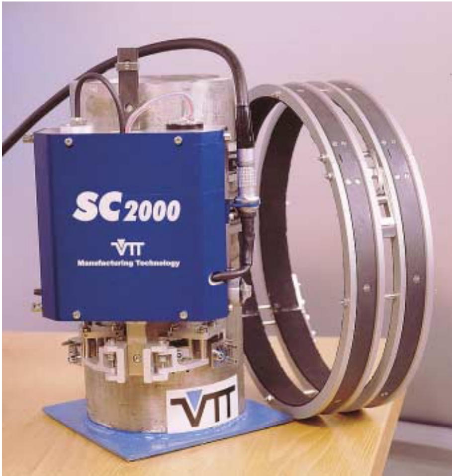
Figure 8. SC2000 scanner for mechanised ultrasonic inspection of pipings.
