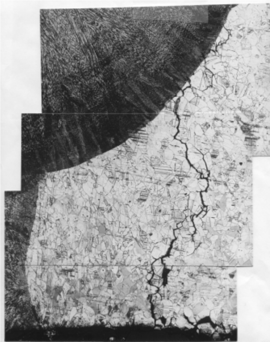
Figure 2. IGSCC in sensitised AISI 304-type stainless steel.
