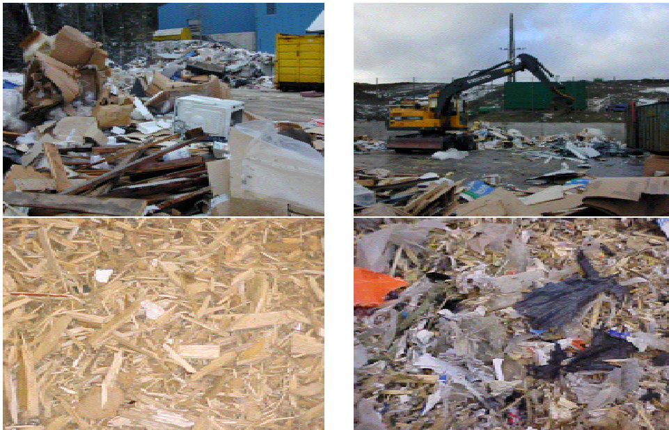
Figure 3. Fuel treatment: upper left: industrial waste, upper right: removal of large pieces, lower left: crushed recovered wood, lower right: pre-treated fuel.
