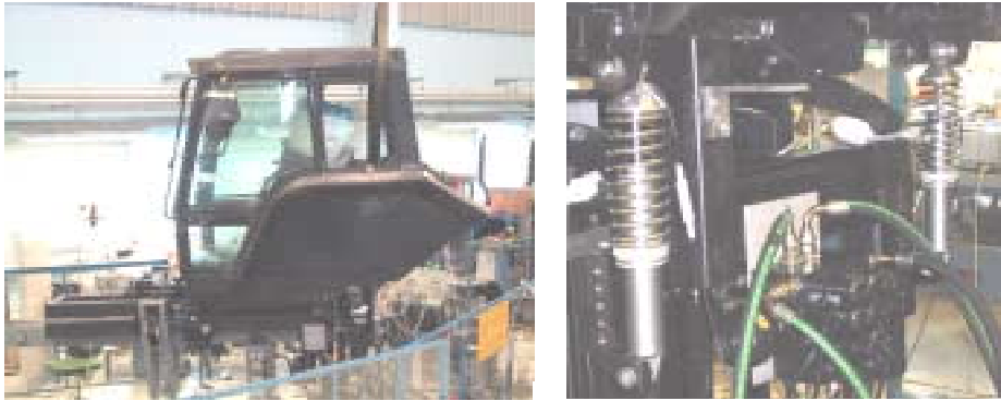
Figure 7. Tractor cabin test bench (left) and the two MR damper/coil spring sets installed between the cabin and the bench. The hydraulic hoses and the associated block are not part of this experiment.
