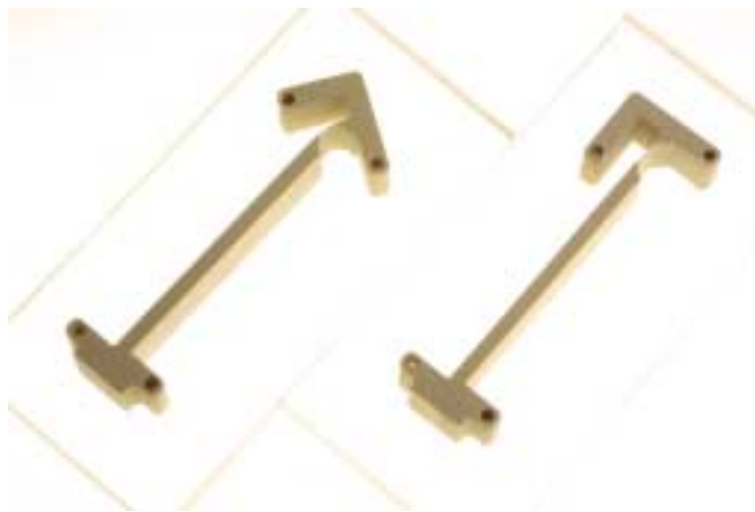
Figure 2. Both modules have joints that can bend 45° elastically.
