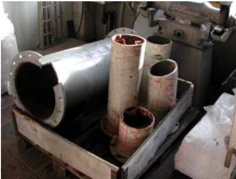
Figure 1. Flanged seawater pipes having outside diameter of 220 mm and 420 mm were examined.
