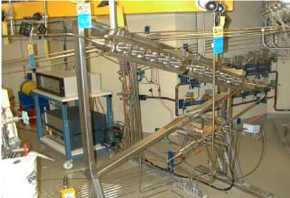
Figure 1. The flow-through cells with high temperature water chemistry sensors and 80 material samples at Loviisa 1 plant.
