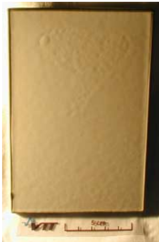
Figure 4. Oil smear on the steel surface destroys the coating in the immersion test. Oil smear area can be seen in the upper part of the specimen where also one large blister is seen.
