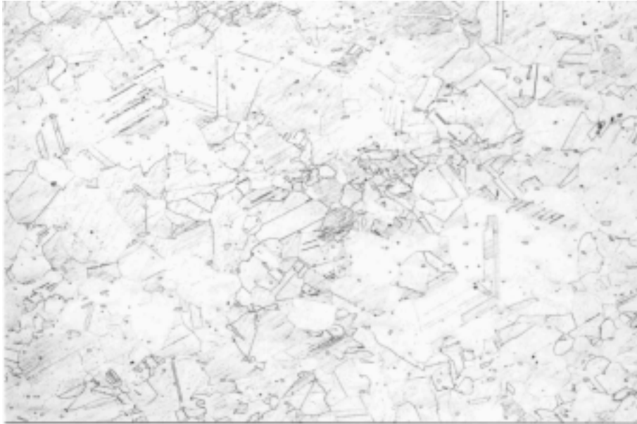
Figure 15. Optical micrograph of the lower fluence material, initially calculated 1.5 dpa. Grain size ASTM 4–4.5. (100X).
