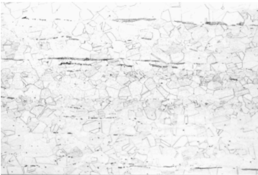
Figure 16. Optical micrograph of the higher fluence material, initially calculated 4 dpa. Grain size ASTM 5. (100X).
