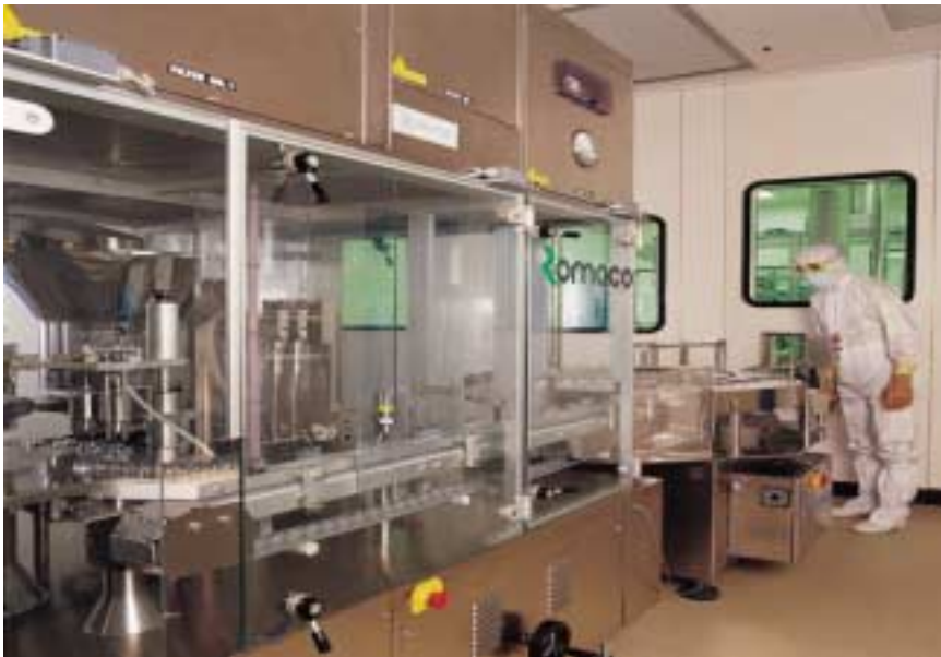
Figure 3. A typical pharmaceutical filling machine showing complex surfaces and the use of different materials.
