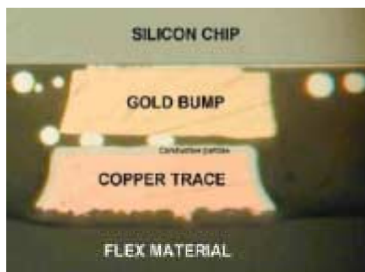
Figure 3. Cross section of ACA-contact.
