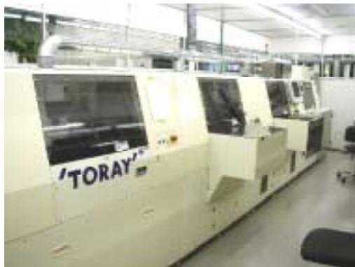
Figure 5. ACA production line protected with class 10 000 clean room.
